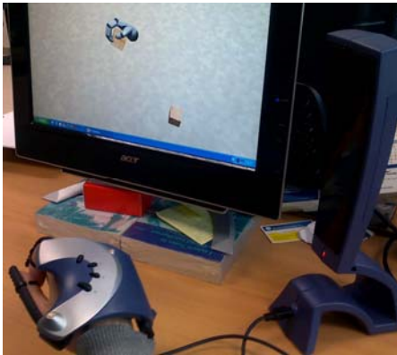
Fig. 4. Detail of the P5 data glove during a simple test: “grasp a virtual cube”.
